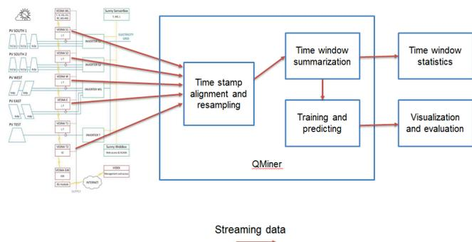
Figure 1. Online PV current production forecast - system overview
