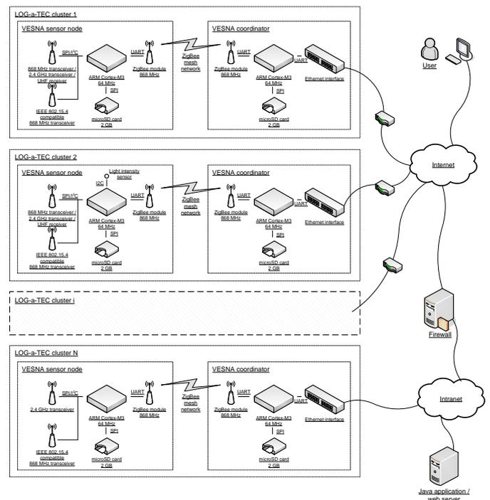
Fig. 1. A logical block diagram of LOG-a-TEC experimental sensor network
