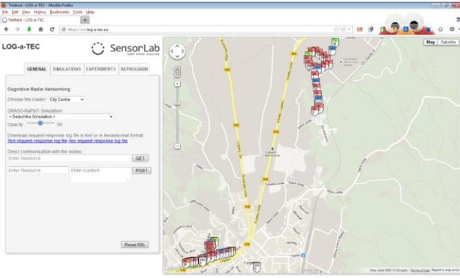
Fig. 2. Web interface to access experimental sensor network LOG-a-TEC provided with a readily available GPRS module. A logical block diagram of the LOG-a-TEC sensor network and its connections with the control application is shown in Fig. 1.
