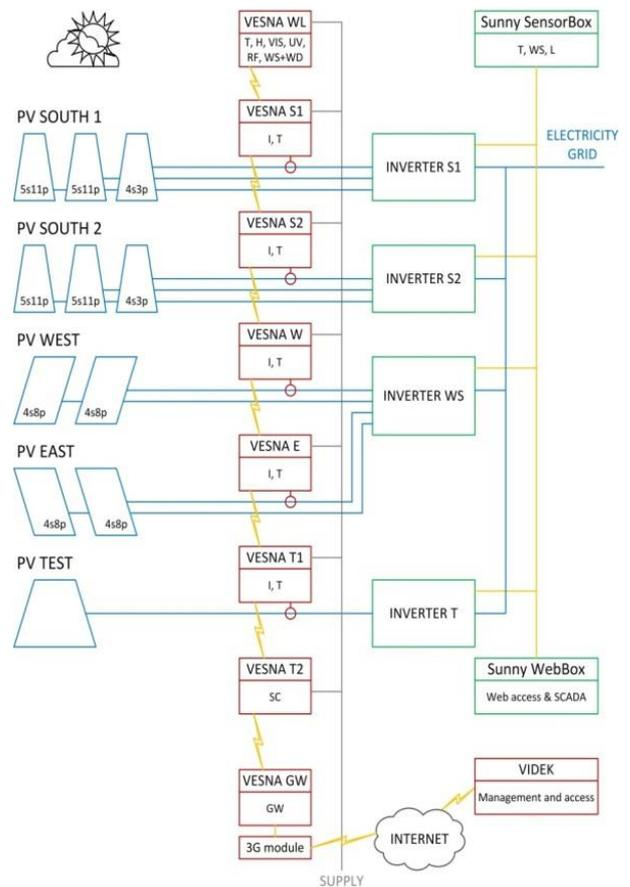
Fig. 5. VESNA based WSN for real time monitoring of PV system
